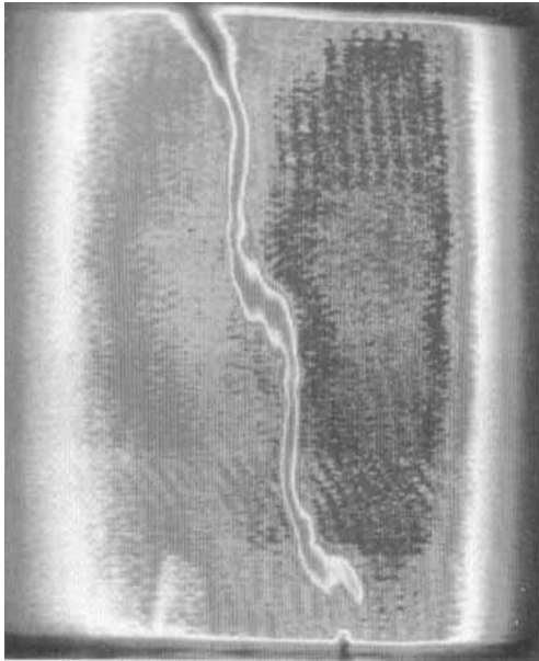
FIGURE 3. (a) Dyeline pattern for \omega = 1.36 , \theta = 1^\circ . The time is 6.5 \pm 0.3 non-dimensionally or 3.90 s on the videotape record. Image enhancement as figure 2; vertical stripes in the background are due to an unavoidable enhancement of the moulded-plastic light diffusers behind the tank. (b) As (a) but time is 10.0 \pm 0.3 non-dimensionally or 6.00 s on the videotape record.
